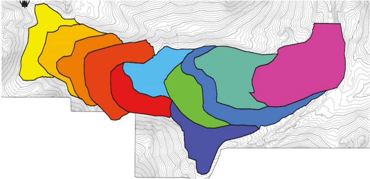
Figure 3: Example of heap leach pile in plan view. Each colour represents a different operational phase
