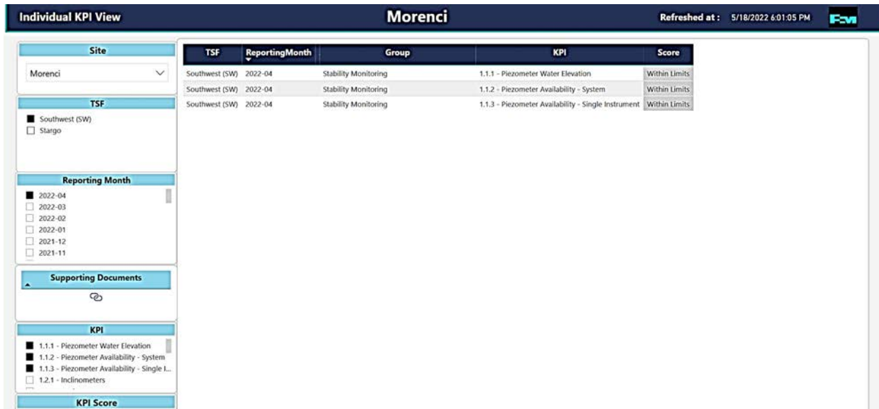
Figure 2: Power BI showing a summary of phreatic surface KPI score for a particular month
