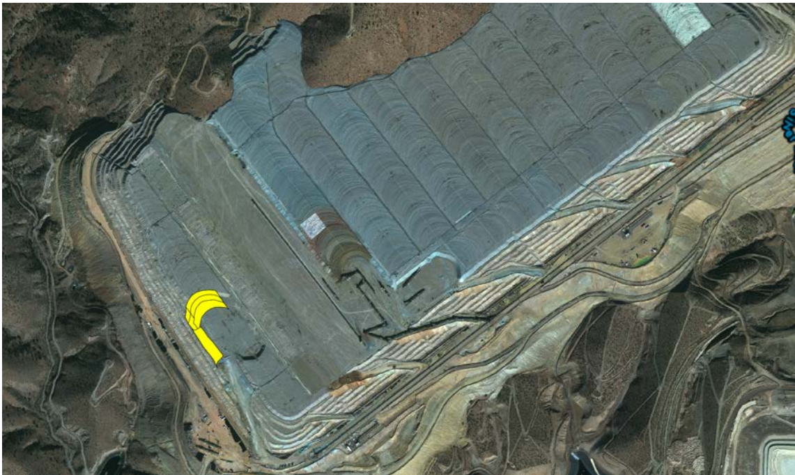
Figure 3: Shape (yellow), showing high clay content of material stacked on a particular day
