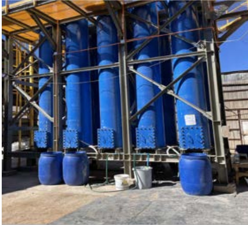
Heap leach column set-up
