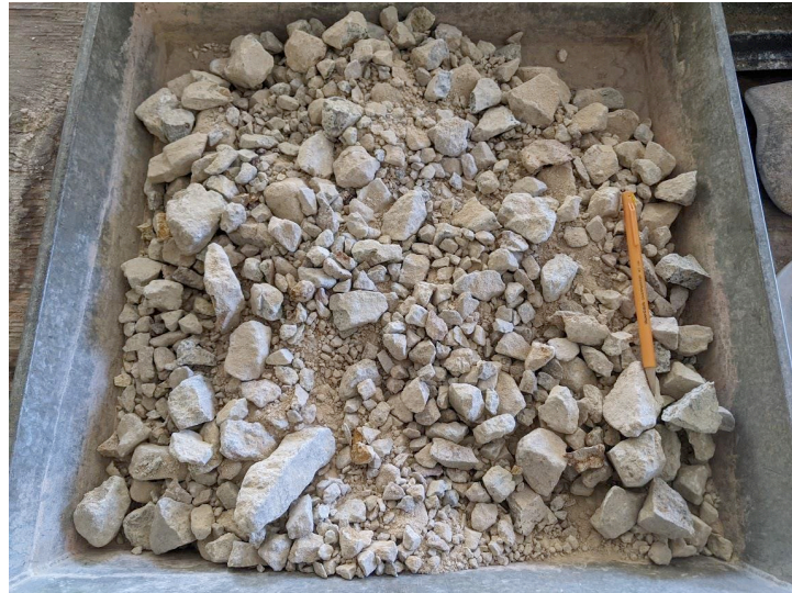
Figure 5: Overliner material used in large-scale puncture test
