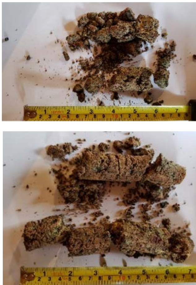
Figure 6: Condition of sample at 5 m depth (top), and sample at 10 m depth (bottom)
