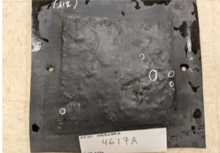
Figure 4: 2 mm HDPE geomembrane after puncture test
