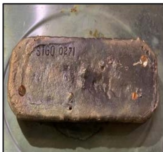
Figure 4: Smelted copper out of waste solution
