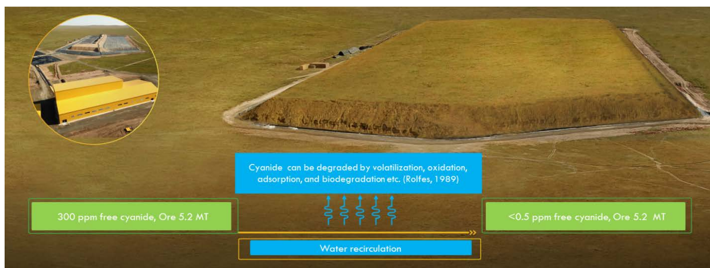
Figure 5: Conceptual plan for heap leach pad closure
