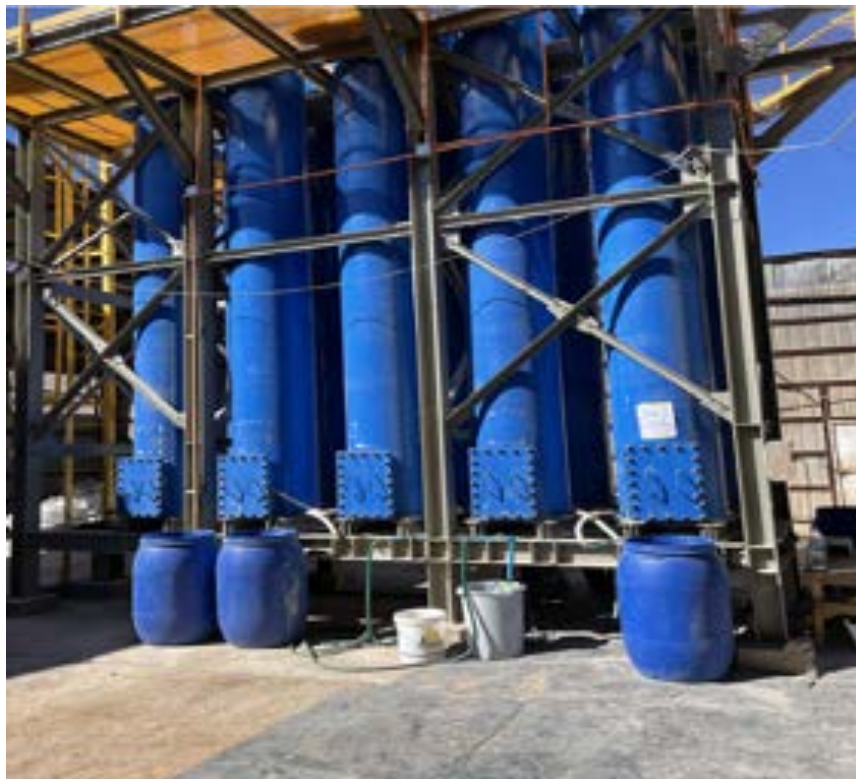
Heap leach column set-up
