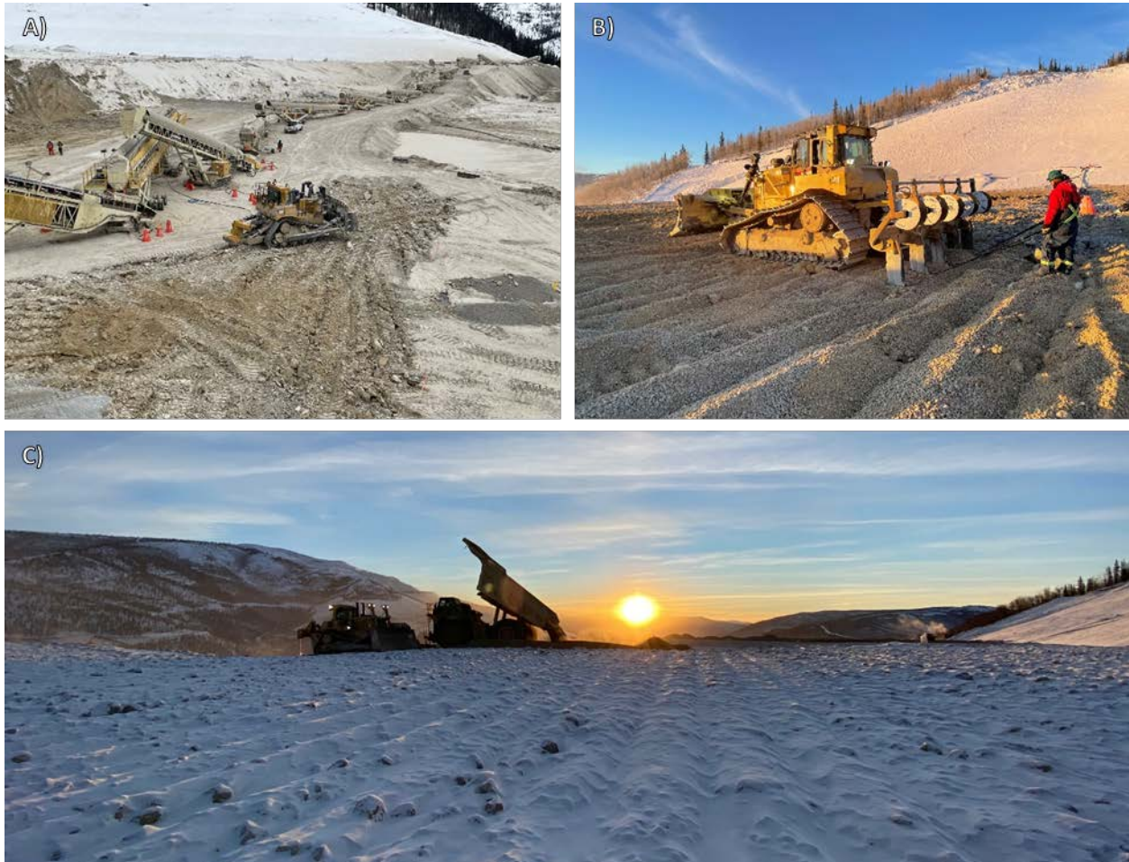
Figure 4: Leaching operations at Victoria Gold Corp. A) Cross ripping ahead of advancing stacking B) Installation of buried drip lines C) Leaching area
